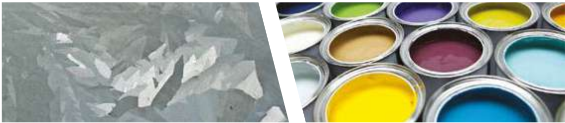
Typical pattern of hot-dip galvanized steel
